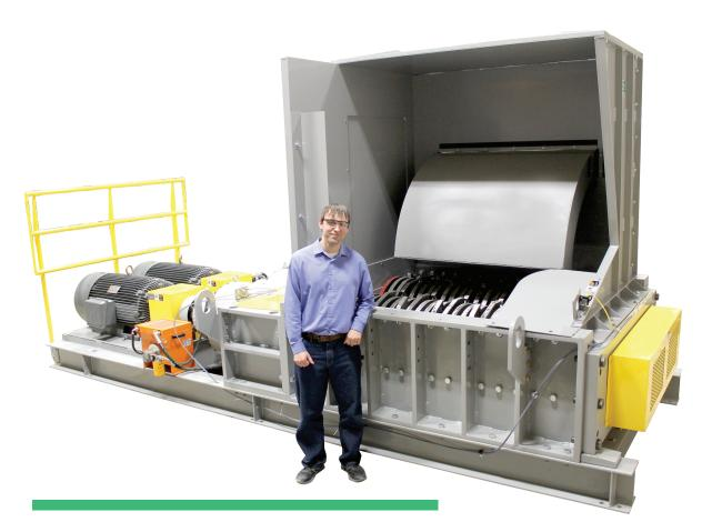
Pictured above is Karl Larsen, Lead Engineer for Amos Mfg. Behind him is a one-of-a-kind 500 HP dual shaft shredder. It features extra seals, special combers, and variable frequency drives on each dual motor shaft. This shredder's user-friendly design also offers the flexibility of adding other heavy duty equipment in the future. This shredder can process up to 15 tons of various plastic materials per hour.
